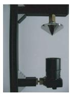
Figure 10: Catadioptric system mounting the camera and the conical mirror.
